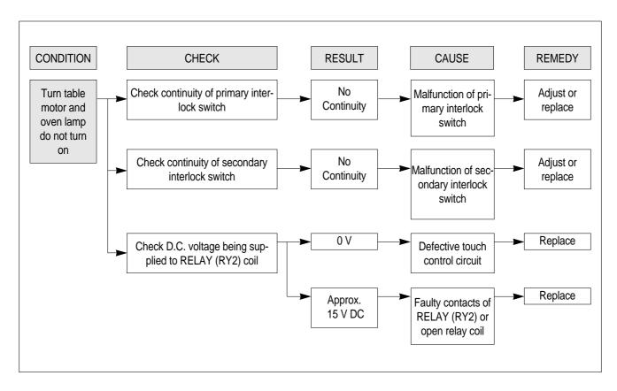
(TROUBLE 3) No microwave oscillation even though fan motor rotates.
